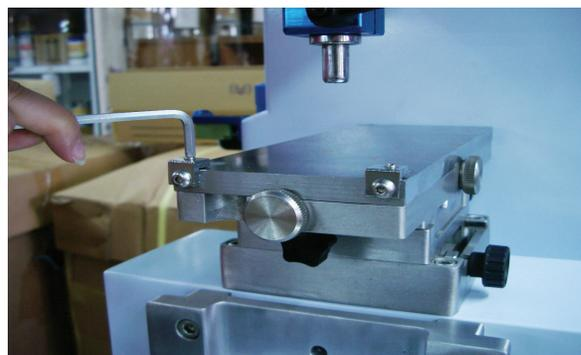
2. Loosen the 2 small locking screws on top front of each base plate by a hex key wrench. Then, put the thin steel plate with the ink cup (make up as per picture at left) on top of the base plate and lock back. Make sure that the etched plate is tightly locked under the 2 small clips.
