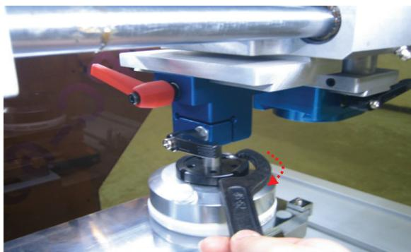
5. You can use the spanner to adjust the distance between the magnet and the steel plate. If turning the ink cup clockwise, the magnetic will be stronger between the ink cup and steel plate. While turning it anti-clockwise, the magnetic will be weaker.
