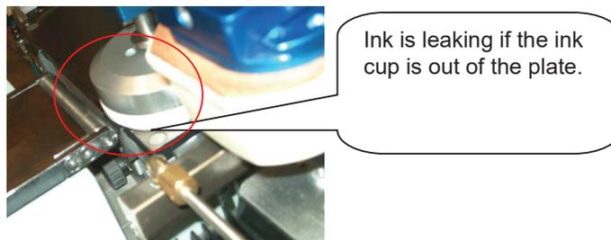
The following diagrams are indicating the correct position of ink cup and plate:
