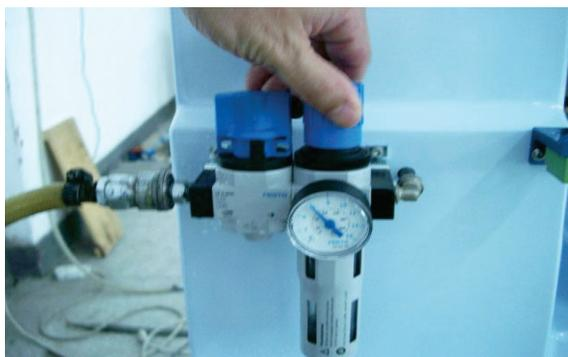
3. Pull up and twist the pressure knob to get the pressure around 5 – 6.5 bar. Press down the knob when you get the desired pressure.
