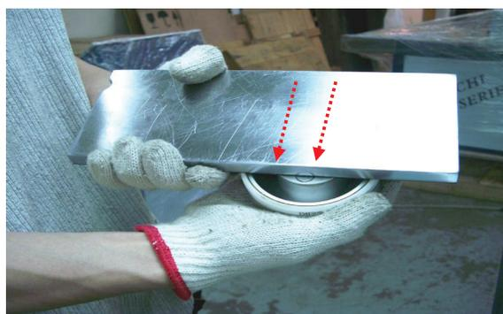
4. If you want to take out the ink cup from the etched plate, make sure that the cup is facing up and the etched plate is on top of it in order to prevent ink leaking. Then, slide the cup to the side of the thin steel plate and finally slide out from the plate. Never try to forcefully pull out the ink cup. This will damage the thin steel plate and the ceramic cup ring.
