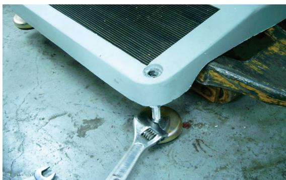
1. If your machine is with a stand, install the leveling foot pads through the foot pad holes, preferably in an air-conditioned clean room with temperature around 18-28°C. Otherwise, you can simply put the machine on a table.
