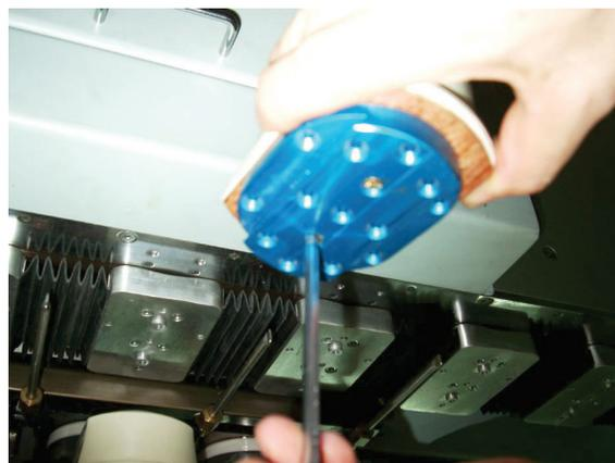
To attach the printing pad, take out the pad holding plate as shown on left and then attach the pad under the plate by using a screwdriver. There is a M6 hole in the centre of the pad holding plate. If your pad is built-in with a M6 screw, you can simply put your pad through this hole.
