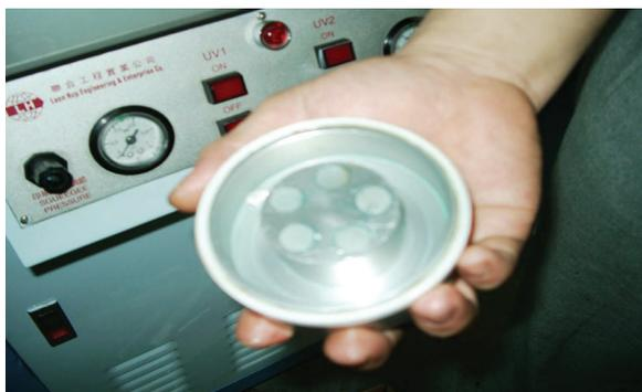
1. Pour ink into the ink cup. Cover the ink cup with the cliché (i.e. etched thin steel plate or polymer plate). Please make sure that the etched side should be facing the cup. Now, you can reverse the ink cup with the plate under it.
